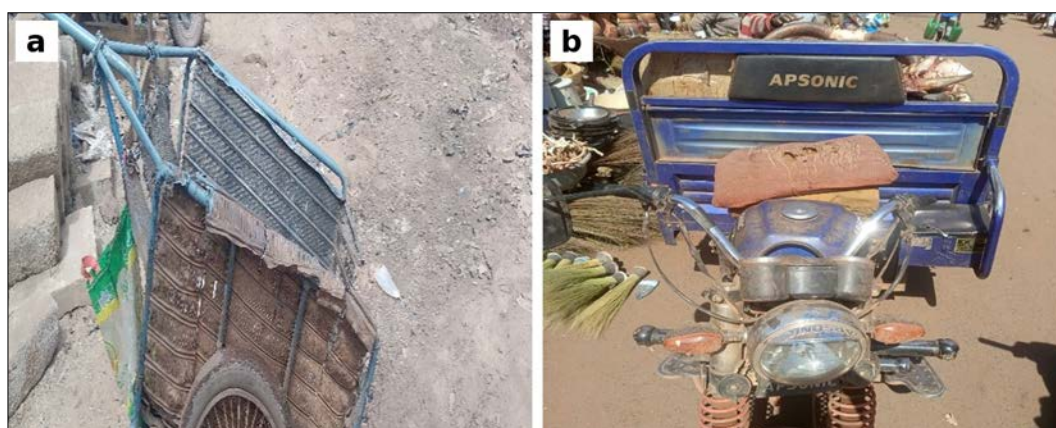
Fig 5: Means of collecting market waste: (a) handcart; (b) motorised tricycle
